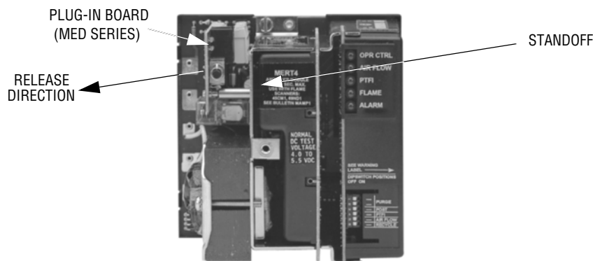
FIGURE 4. PLUG-IN BOARD LOCATION AND INSTALLATION
